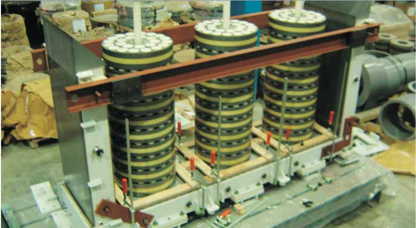
An assembled 5-limb reactor core, upper yoke and fixed threaded bolts.
